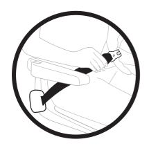
To fasten the seat belt, pull out the belt and insert the clasp into the buckle. A positive click should be heard, indicating that the lock has engaged properly.
