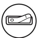
2. **Switch off the battery isolation on the carriage.** (Located next to the key and display on the carriage unit)
