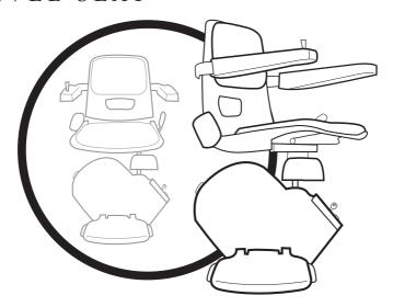
When the unit reaches the upper end of the track, it will stop automatically.
