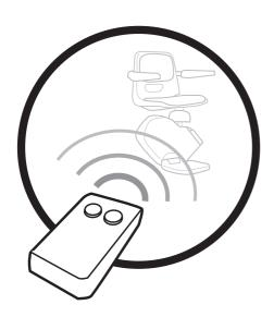
The unit may also be operated with the remote control handset. There are two buttons on the handset.
