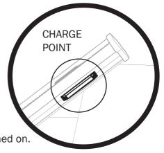
On a STANDARD TRACK, the correct positions are at the top or bottom where the unit stops automatically. At these positions, the unit receives a power supply from the mains / transformer that allows the unit to recharge its internal batteries.
