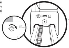
The display panel, positioned near the key switch, will indicate 'A1'. If the display is not indicating 'A1', please check the *DIGITAL DISPLAY CODES* on pages 17-20.
